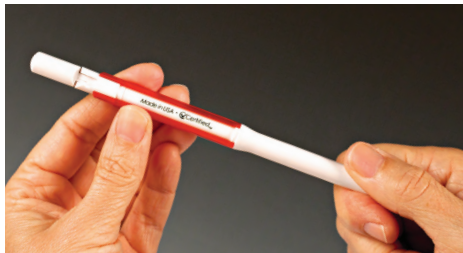
Grip Aesthesio® Evaluator protective sleeve with one hand and rotate the handle with the other.
