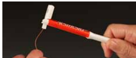
Ready for testing. Return filament to channel and rotate sleeve closed when complete.
