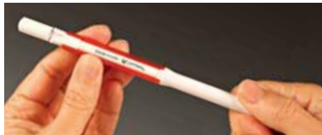
Grip Aesthesio ® Evaluator protective sleeve with one hand and rotate the handle with the other.
